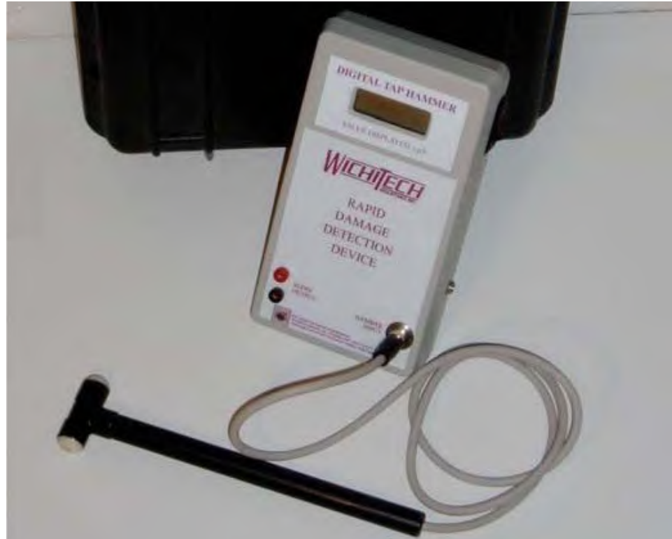
Figure 7.3.6 Electronic Tap Testing Device
